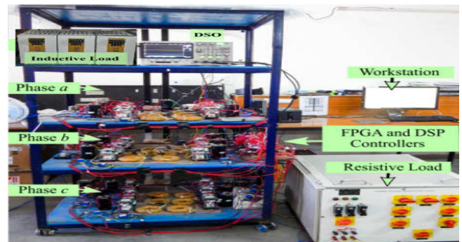
Fig. 11. Experimental set-up of 3- \phi MMC.
