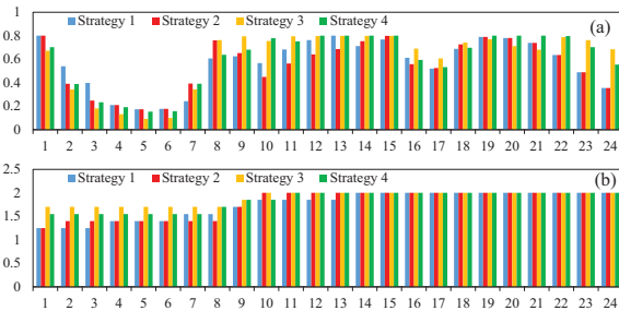
Fig. 8. Total reactive power injection from (a) BESSs (b)CBs.
