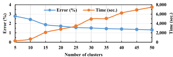
Fig. 2. Error in the objective function and computational time with a different number of clusters.
